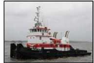
at 1,800RPM, driving three fixed pitch propellers via CAT 5202 3.42:1 gears.
