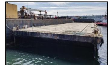
specialized cargoes. The barge had 27' long bow & stern rakes with twin towing skegs aft, a breakwater forward plus a new concrete wear deck. One longitudinal and five transverse bulkheads formed 12 watertight compartments. The barge was classed ABS A1, Barge, Unrestricted Service and laid up in active class at the time of the sale. Marcon International acted as sole broker. Over the last 37 years, Marcon has sold 232 inland and ocean deck barges totaling about 1,070,000dwt capacity.
