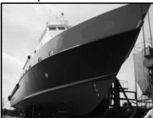
Patterson, Louisiana. She is classed ABS + A1, HSC Crewboat + AMS and USCG certified under Subchapter T. Capacity is 193mt deadweight including deck cargo of 153mt on 1,764ft<sup>2</sup> clear deck. Vessel is powered by four Cummins KTA38M2s developing a total of 5,400BHP at 1,950RPM driving 4 - 44" x 48" fixed pitch propellers providing a speed of 22-27 knots. Vessel has quarters for 8 in 5 cabins and passenger seating for 80. Marcon acted as sole broker in the transaction.
