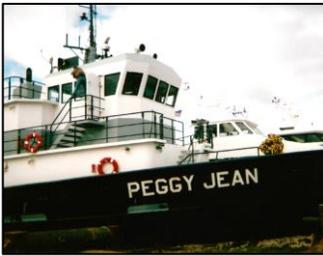
KTA38-M0s developing a total of 1,700BHP at 1,800RPM and fitted with a 300HP 36" Thrustmaster bow thruster. She is capable of carrying 350 long ton cargo on a 80' x 32' clear deck aft and has tankage for 115,000g potable water, 90,000g fuel and 700g lube oil. Accommodations include 18 berths in six cabins.
