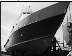
Patterson, Louisiana. She is classed ABS + A1, HSC Crewboat + AMS and USCG certified under Subchapter T. Capacity is 193mt deadweight including deck cargo of 153mt on 1,764ft2 clear deck. Vessel is powered by four Cummins
