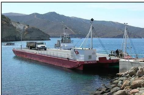
The U.S. flag, ABS coastal loadline, deck barge “*Islander*” was sold between U.S. West Coast interests. The 128’ x 38’ x 7’8” barge was built in 1964 at Southern Oregon Marine, carries around 532 tonnes of cargo and is fitted with a 26’ long x 12.5’ – 18’ wide aft ramp. Until recent times, “*Islander*” served as a freight barge to Santa Catalina Island off the southern Californian coast, but was deemed excess to requirements after the contract changed hands. New owner intends to convert the
