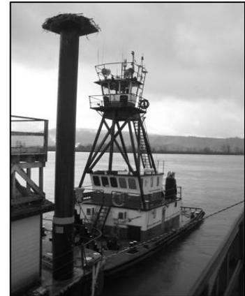
1-1/8" wire plus two hydraulic Gearmatic bow winches and capable of pushing 4,000 ton rock and 4,500 ton chip barges plus tending dredging projects. Her elevated wheelhouse provides the operator with excellent vision. All four hydraulic winches can be operated from both the upper and lower wheelhouses. Marcon acted as sole broker and has handled a number of sales and purchases for both buyer and seller in the past.
