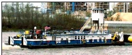
567Cs totaling 3,200BHP which were installed in 1968. She has Falk LST 2.48:1 gears and 4-blade stainless steel props on 8” shafts, two steering and four flanking rudders. The boat is also fitted with a retractable pilothouse with 17.5’ of lift and push knees both fore and aft. Accommodations are provided for nine crew. Most of the “*Kristin Lee*
