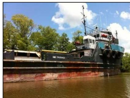
The vessel is powered by two CAT D399TA main engines for a total of 2,250BHP at 1,225RPM, driving two fixed props. Her speed is about 12 knots. She has an 89' x 21' clear deck and can carry 4,000BBL of liquid mud. Air conditioned accommodations are fitted for up to 22 persons.
