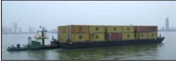
File: DB15440 Deck Barge - Coastal: 154.0' loa x 40.6' beam x 8.2' depth x 0.90' light draft x 6.56' loaded draft. Built in 2008. Colombia flag. Dwt: 950T. Deck Load: 6MT/m 2 . Holds 60 TEU or 30 FEU. Caribbean.
