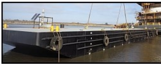
File: DB19030 Spud Barge - Inland: 190.0' loa x 30.5' beam x 9.0' depth. Rebuilt: 2017. U.S. flag. Class: Not classed. Dwt: 270st. 190' x 30' clear deck. Deck Load: 2,000lb/ft 2 . Deck/spud barge converted from pontoon barge in 2017. Two 45' x 20" spuds, manual lift with crane. External spud wells. In 2017, new anodes, sandblasted and painted inside and out. Reportedly in like-new condition. Photos, drawings and UT reports upon request. U.S. Gulf Coast.
