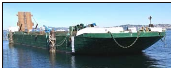
File: DB20058 Deck Barge - Ocean: 200.0' loa x 198.5' lbp x 54.0' beam x 13.0' depth x 2.00' light draft x 10.45' loaded draft. Built in 1967 by Gunderson, Portland, OR. U.S. flag. GRT: 952. NRT: 285. ABS Loadline exp Aug 2022. USCG COI. Exp. Feb 2026. Dwt: 2,500T. Rakes: Double. Bulkheads: 1 long 'l / 4 transv. Capacity: 19,783bbl. Tanks: 7. Crane: Hose boom. Gensets: 1 - 2kW. Ex-Single skin petroleum barge. Spoon bow. Tow sklegs aft. Breakwater (38") forward. TPI 24.5ST. Originally built as deck barge, then put into black oil service before being sold & converted back to deck service. 6" timber wear deck. 18' x 30' stern ramp. U.S. Northwest.
