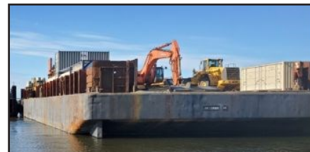
File: DB24971 Deck Barge - Ocean: 250.1' loa x 72.1' beam x 15.5' depth x 12.75' loaded draft. Built in 1988 by Galveston SY; Galveston, TX. U.S. flag. GRT/NRT: 1,942. ABS Loadline (on drydock now for renewal). Dwt: 5,450T. Lt Displ: 970T. Deck Cargo: 5,450ST. Deck Load: 1,500lb/ft 2 . Rakes: Double. Bulkheads: 2 long'l / 6 transv. Watertight Compartments: 21. Towing sklegs aft. Interior not coated. 8' bin walls and new concrete wear deck installed Q1 2016. Extensive internal steel work also performed in 2017-2018. Portable 50' x 5' twin ramps available for additional charge. Not officially on the market, but owner will consider a sale. On drydock now (March 2022) for maintenance and renewal of loadline. Expected to be completed in a few months. U.S. Northwest.
