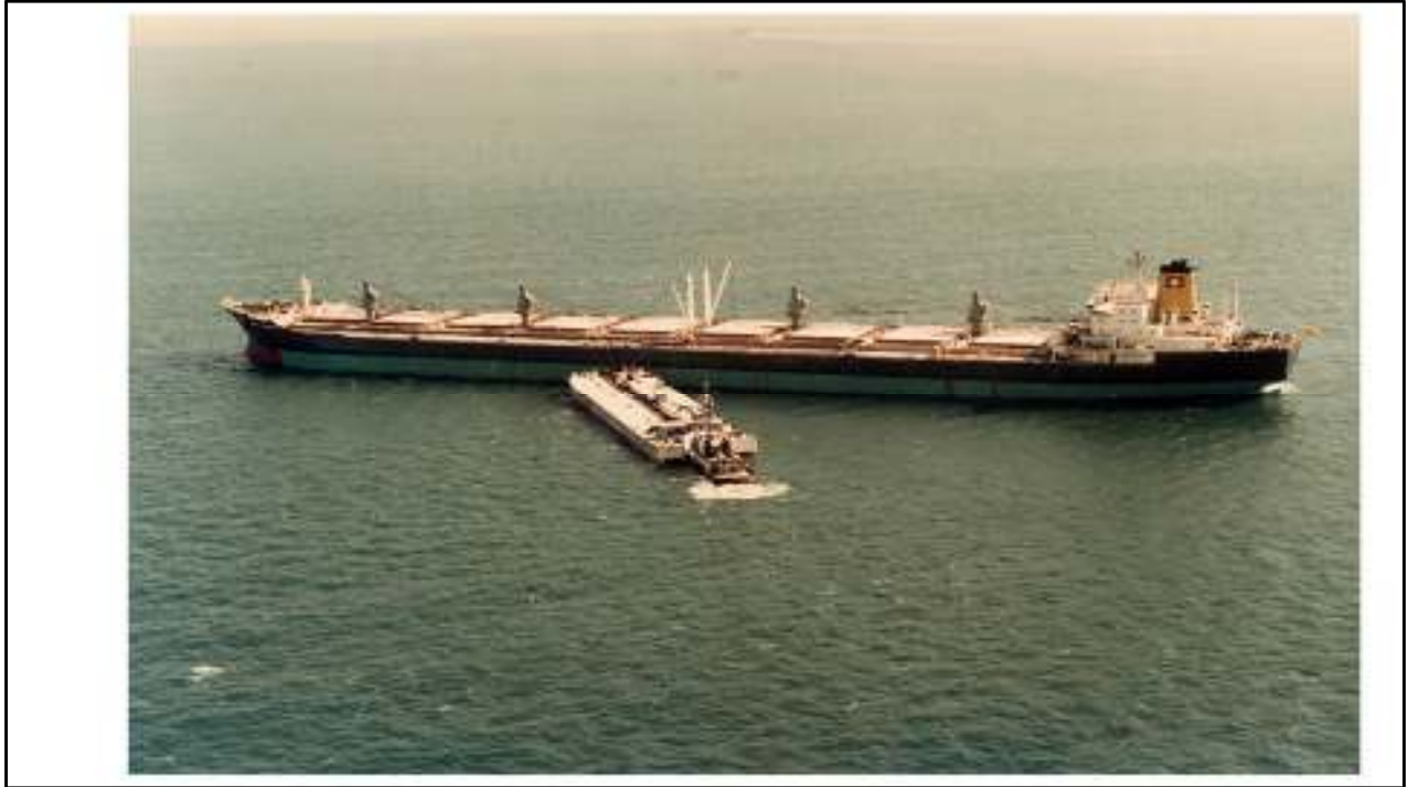
Tug RENE J CHERAMIE towing a barge with a capacity of 65,000 barrels lightering ships loaded with Crude Oil. This job was pre LOOP / Louisiana Offshore Oil Port.
