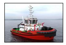
and deep-sea towage services. The tug is fitted with two Caterpillar/3516E main engines, each developing 2,100kW at 1,600rpm and with two Kongsberg/US 255S FP thrusters. It is also equipped with FiFi 1 class fire-fighting system, capable also of providing oil recovery and escort services.
