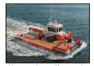
vessel maximum maneuverability. The two strong HEILA marine deck cranes fwd and aft with a maximum lift capacity of 7.70mt at 16.39 meters and 7.85mt at 14.42 meters, the double drum towing/anchor handling winch of 50mt (pull), a 10 and 12 metric tons tugger winches, option for spud poles two Ø 610mm and a maximum clear deck area, makes the vessel more than multifunctional and definitely one of a kind. Options for seabed levelling/dredging operations are an Aft Portal A-frame for ploughing.
