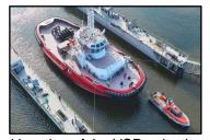
emissions are reduced with an IMO Tier III after-treatment installation. Due to the forward location of the VSP units the LNG tank hold is located aft of the engine room, providing separation of the gas system and any associated hazardous areas from the accommodation block. Particulars of the TRAktor V3900-DF are as follows: Length Overall: 39.0m; Beam, Moulded: 15.0m; Depth, Moulded: 6.0m; LNG Capacity: 40m3; Diesel Oil Capacity: 164m3; Power: 2 x 3,000kW; Bollard Pull (predicted): 80mt.
