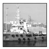
File: <u>TG31012</u> Tug - Twin Screw: 121.4' loa x 37.4' beam x 16.2' depth x 13.30' loaded draft. Built in 2007 by SE Asia shipyard. Malaysia flag. GRT: 467. NKK NS\*(TUG/FFV1/AHV) MNS\* MPP, LSA, RCF, AFS Exp. April 2022; Next DD due Oct 2020. Laid-up. FO: 312m3. Main Engines: 2 x CAT 3512B-TA total **3,150BHP**. 2 - FP props. **Bollard Pull: 47mt**. Gensets: 1 - 150kW / Cummins 6CTA8.3. AirCon. Galley. Two anchor handling sister tugs available for sale. **Southeast Asia**.
