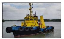
Marcon can report it closed on the sale of the twin screw, ocean going tug "San Felipe" from SAAM Towage to its new South American owners. Built in 1996 at President Marine Pte, Singapore; the 2,800BHP unit measures 95' x 28' x 13' and is powered by twin Yanmar T240-ET main engines. The vessel is surveyed under Lloyds Register Class. The tug is being repositioned to the new owner's location and will eventually be renamed. Marcon was the sole broker in the transaction.
