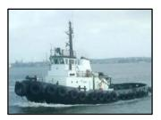
**File:** <u>TG35103</u> **Tug - Twin Screw:** 105.0' loa x 32.0' beam x 16.9' depth x 15.25' loaded draft. Built in 1972 by Carrington Slipways Pty Ltd; Australia. Foreign flag. GRT: 268. LR disclassed. Laid-up. Winch: Tow hook. Main Engines: 2 x Blackstone ESL16MK2 total **3,500BHP**. 2 - 4-blade FP props. Kort nozzles. **Bollard Pull: 44T**. Gensets: 2 - 40kW 415vAC 50Hz. Laid-up. **South America East Coast.**
