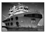
D(M), 1 - 150kW / Cummins 50Hz AC. **FiFi 1**. 1,200/300m3/h water/foam remote joystick monitors. 42 berths in 12 cabins. Handy-sized anchor handling tug. 120T SWL stern roller. 200T SWL Karm Fork & tow pins 2 - 10T tuggers and 2 - 5T capstans. Foam: 16m3. CO2 system: 6 - 45kg tanks. Dispersant: 19m3. Sewage treatment: 2.1m3/d. 6 person rigid rescue boat. Four Crowcon H2S sensors. **Southeast Asia**.
