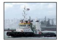
File: <u>TG28193</u> Tug - Twin Screw: 95.1' loa x 28.2' beam x 13.5' depth x 11.80' loaded draft. Built in 1995 by President Marine Pte.; Singapore. Panama flag. GRT: 223. LR 100A1 LMC - Exp. Apr 2025. Dwt: 164mt. Light Disp.: 265mt. FO: 96.4m3. FW: 38m3. Winch: Tow Hook. Main Engines: 2 x Yanmar T240-ET total **2,800BHP**. 2 - Bronze FP props. **Bollard Pull: 39T**. Gensets: 2 - 60kW / Leroy GM6-71 380vAC 50Hz. Quarters: 7 crew. **South America West Coast. Q4 2023**.
