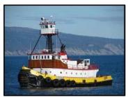
10' stern roller; six rudders, 85,000g liq. Capacity can be divided into F.O. & water. No load line necessary, due to low GRT. Anchor handling. **Caribbean.**
