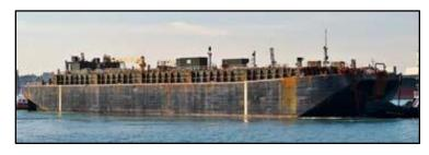
4,500bph, Byron Jackson LS-12, 4 Stage. 1 - 5,000lb anchors. Windlass: 1 - Hatlapa 100 hydraulic. Crane: 2 - EBI C-10-B (4,000lb). Gensets: 2 - CAT3406 (cargo pump); 1 - 45kW John Deere. Double hull, all welded steel construction. All tanks are coated. (National NC-600). 2" cargo stripping system. Bergen tank radar gauging system / high level and overfill alarm system. Raised trunk. TPI at Loadline = 57.58LT. **U.S. Northwest.**
