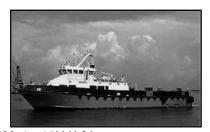
10m3/h, Bilge/BW: 26m3/h, General: 26m3/h. Gensets: 2 - 52kW/Perkins 4 SabreTGM, 1 - 10kVA/Yanmar 380/415vAC 50Hz 3Ph. Firefighting: 1,200m3/h pump & Ekhart monitor. Gyro. Autopilot. Radars: 2. GPS. Fathometer. SSB. VHF. Navtex. Satcom. Quarters: 10 persons. AirCon. **Passengers: 60 seats**. Aluminum hull crew / fast utility vessel. Lifesaving & firefighting as per SOLAS requirements. 1 hospital. **Southeast Asia.**
