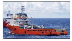
2 - CP props. 1- 883kW CP (f) thruster; 2- CP (a) thruster. Bowthruster 883kW. **Bollard Pull: 190mt**. Speed about 15-17kn. Gensets: 2 - 3,000kVA shaft; 1 - 1,668kVA aux; 1 - 488kVA emer. GPS. Quarters: 28 (12-1, 2-4, 4-2). AirCon. Galley. UT 712L design. AHTS. 16 marine crew. 114.8" (35.0m) air draft. Three mess/rec rooms. 4 - 98m3 rig chain lockers. Two roll reduction tanks. RR ICON DP 2 positioning system. Currently in lay-up. **Europe Northern.**
