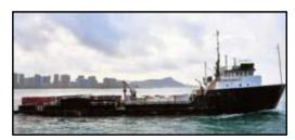
AirCon. Galley. Passengers: 12. ITC - 704G / 211 N. Container capacity 30 TEUs / 12 FEUs (6 reefers). Bowthruster engines CAT 3406. Vessel set up for project cargo, heavy equipment / vehicles, roll-on roll-off (no fixed ramp), load-on load-off, containers / refrigerated containers, ISO containers (liquid cargo), or palletized cargo. Capable of ship-to-ship and ship-to-shore transfers of fuel and potable water. **South Pacific. Prompt.**
