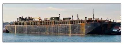
File: TB81833 Double Hull Tank Barge - Ocean: 332.0' loa x 316.4' lbp x 74.0' beam x 25.0' depth x 4.50' light draft x 22.10' loaded draft. Built in 2002 by Friede Goldman Halter; Moss Point, MS. U.S. flag. GRT: 5,790. NRT: 3,846. Class: ABS+A1, Oil Tank Barge Unrestricted. USCG COI Grade "A" and Lower. SS due Aug 2022. Dwt: 11,964lt. Lt Displ: 1,860lt. Rakes: Double. Bulkheads: 6 transv / 1 long'l. Capacity: 81,751bbl. Tanks:
