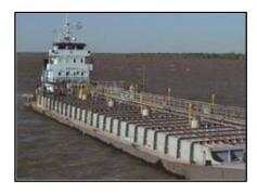
**File: TB28129 Double Hull Tank Barge - Inland:** 297.5' loa x 59.0' beam x 15.4' depth x 11.60' loaded draft. Built in 1979 by US Shipyard. **Rebuilt: 2011**. Foreign flag. GRT: 1,538. NRT: 1,461. Class: RINA C + barge-oil product; inland waterways 2. **Dwt: 4,420mt. Capacity: 27,625bbl**. Tanks: 8. Double Hull retrofit in July 2011. Cargo capacity 5,054m3 at 100%. Suitable for the transport of petroleum distillates with a flash point lower than 60 degrees C. **South America East Coast.**
