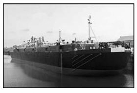
hydraulic drive & pump system. Vapor Recovery system. Yokohama fender slides port fore & aft. Emergency tow wire. Panama chocks. Dry docked, painted & all certificates freshly renewed late 2018, including second five year Special Survey, etc. ITC Tonnage: 5,813G / 3,914N. Compatible tug side of JAK system from former tug may be made available for installation on new tug. Owner will entertain offers. **U.S. Gulf Coast.**
