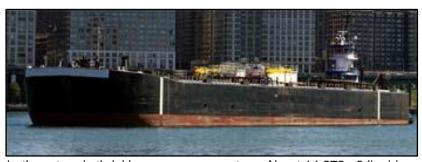
discharge 4,300BPH. Double hull. Seven tanks both port and stbd. Vapor recovery system. About 14,279m3 liquid capacity. Oil - F.P. 60 deg C or less and chemicals. **U.S. East Coast.**
