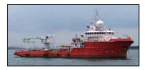
**111.9mt.** Speed about 12-13.5kn. Gensets: 2 - 370kW, 2 - 1,800kW 440vAC 60Hz; 1-172kW emer. FiFi-1. 1,200m3/h @ 11 bar; 15m3 foam. Quarters: 60 persons. Conan Wu AHTS / light OCV. 12 marine crew. Shark jaws; towing pins; and rig chain lockers. **Kongsberg KPOS DP-21 +cJoy** positioning system. Laid up. **Southeast Asia.**
