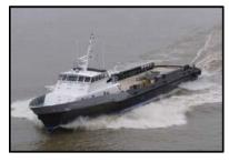
File: CB16234 Crew Boat: 162.0' loa x 29.5' beam x 11.6' depth x 8.00' loaded draft. Built in 2004 by Breaux Bay Craft. U.S. flag. GRT: 98. ABS Loadline. USCG COI. Laid-up. 250LT on 100' x 25' clear deck. FO: 16,560g. FW: 900g. DW: 29,580g. Main Engines: 4 x CAT 3512B total 6,500BHP. 4 - FP props. Bowthruster 375HP. Speed about 23-27kn on 275-350gph. Gensets: 2 - 160kW / CAT 3306, 240v, 60Hz. Quarters: 8 persons / 4 cabins. AirCon. Galley. Passengers: 72. Owner is a keen Seller. U.S. Gulf Coast.
