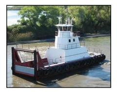
**File: TP16070 Push Boat:** 70.0' loa x 26.0' beam x 7.0' depth. Built in 1971 by Inland Marine Const.; Evansville. U.S. flag. GRT: 150. Main Engines: 2 x CAT 3508 total 1,600BHP. Repowered 2002. Inland river pushboat. Retractable wheelhouse. Needs repairs. **U.S. Midwest.**
