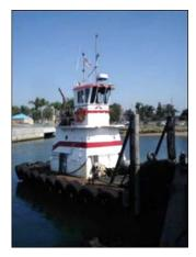
**File: TP05032 Push Boat:** 32.0' loa x 14.5' beam x 7.0' depth x 3.00' loaded draft. Built in 1988 by Clackamas, OR. Rebuilt: 1999. U.S. flag. GRT: 21. FO: 950g. Main Engines: 2 x John Deere 6081 AFM total 500BHP. Last Overhauled: 2005. 2 - FP props. All welded steel hull and house. Connected in 1999 to a push tug. Raised two deck pilot house. Flanking rudders. Vertical push knees. Complete fendering. Major refit mid-2005. Day boat only. **U.S. West Coast.**
