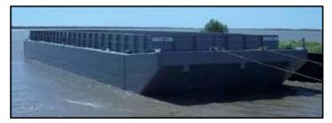
File: HB19552 Double Hull Hopper Barge – Inland (Two Sisters Available): 195.1' loa x 52.6' beam x 11.00' loaded draft. Built in 2013 by Punta Alvear Yard -Ultrapetrol. Foreign flag. Class: RINA Class barge bulk cargo - inland waterways. Dwt: 2,500mt. Hold Capacity: 3,690m3. 1 hold. Steel built dry cargo barge rake type. Height of coaming 1.829mt; Height of double bottom 530mm; Space between frames 740mm; Hold dimensions 54.462m (178.6') x 14.00m (45.9') x 4.944m
