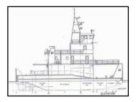
**File: TP13081 Push Boat:** 81.2' loa x 27.1' beam x 11.8' depth x 6.82' loaded draft. Built in 2008 by Astana SA; Argentina. Foreign flag. GRT: 214. Class: BV +I 5 IN (-) + Pusher -DGL IN + MC, exp. 13 Feb 2024. Main Engines: 2 x Volvo Penta total **1,300BHP**. 2 - FP props. Contact Marcon for full details. Vessel reportedly in very good condition, in class and under oil major vetting standards. Just finishing job as of January 2022. **South America East Coast.**
