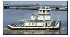
**File: TP08070 Push Boat:** 60.0' loa x 22.0' beam x 9.4' depth x 8.60' loaded draft. Built in 1973 by Phillip Ditta; Harvey, LA. U.S. flag. GRT: 119. FO: 9,500g. FW: 2,500g. Winch: 2 - 20T Nabrico - Hydraulic/Electric. Main Engines: 2 x GM 12V-71 total **680BHP**. 2 - FP props. Gensets: 2 - 30kW / GM3-71. Triple cabin towboat. **Eye level 26'**. **U.S. Gulf Coast.**
