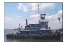
**File: TG11063 Tug - Twin Screw:** 67.0' loa x 24.0' beam x 9.1' depth. Built in 1978 by Terrebone Shipyard; Houma, LA. U.S. flag. GRT: 94. USCG Sub Ch. M - Exp. Sep 2025. FO: 13,000g. FW: 4,500g. Main Engines: 2 x CAT 3412 total 1,100BHP. Speed about 8kn. Gensets: 2 - 30kW GM 3-71 / Delco. Quarters: 6 crew. All welded steel construction Upper Pilot House. **U.S. East Coast.**
