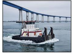
engine produced 500HP @ 1,800RPM through Twin Disc MGX-5136-SC 2.90:1 gears turning two 4 blade 39"x 46" fixed pitch props fitted in Kort nozzles. Pacific Tugboat Service selected the Mitsubishi engines because they provided similar horsepower and engine speed, allowing it to utilize existing shafts and propellers. Southern California
