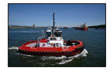
Operating on biofuel, the vessel's fuel-efficient and lower carbon footprint results from a pair of Caterpillar Marine 3516 Tier IV-compliant engines that meet federal mandates and the State of California's environmental regulations. The 6,000BHP Tier IV engines drive two azimuth stern drive thrusters.
