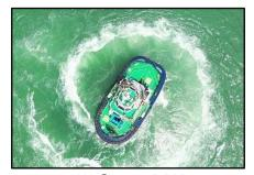
5.05m; Bollard pull: 60mt; Speed: 12 knots (approx.); Main engine: 2 x CAT 3512, 2 x 1,765kW @ 1,800RPM; Propeller: 2 x Kongsberg US205 P20 FP with 2,400mm dia; Fore towing winch: THR Marine EFTW 300 kN; Deck crane: Toimil Marine / T12505M/3 SWL 1.03mt at 10.1m; Generator set: 2 x Caterpillar C4.4 86ekW; Fifi system: 1 x 1,400m3/hr. Pump, 2 x 1,200m3/hr foam / water monitors; Accommodation: 6 persons.
