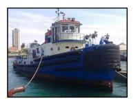
**File: TG30051 Tug - Twin Screw:** 95.9' loa x 28.0' beam x 13.7' depth x 10.50' loaded draft. Built in 1971 by Southern Shipbuilding. Panama flag. GRT: 303. Last Drydocking Fall 2021. Winch: 2 Markey Capstans. Main Engines: 2 x GM 12-645-E2 total 3,000BHP. 2 - FP props. Speed about 12kn. Gensets: 2 - 60kW. **Central America.**
