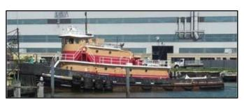
File: TG34121 Tug - Twin Screw: 100.0' loa x 26.8' beam x 9.7' depth x 14.60' loaded draft. Built in 1967 by Main Iron Works; Houma, LA. Rebuilt: 2003. U.S. flag. GRT: 188. ABS Coastwise Loadline. Exp Dec 2016. FO: 38,000g. FW: 1,400g. Winch: Almon Johnson. Wire: 2,000' x 2". Main Engines: 2 x CAT 3516 total 3,420BHP. 2 - 88" x 72" FP props on Stainless steel shafts. Repowered from CAT D398TAs in 1995. Bollard Pull: 75,530lb. Gensets: 2 - 40kW / John Deere120vAC 60Hz. Firefighting: Fixed CO2
