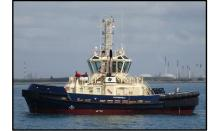
visibility and exceptional visibility to the bow and side fendering. The engine room features an acoustically isolated switchboard room. Trial results were as follows: Bollard pull, ahead: Both "Svitzer Albrolhos" and "Svitzer Wilu" reached beyond the designed bollard pull of 70 tonnes; Free running speed, ahead: 12.8kn.
