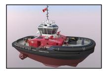
powerful Azimuth Stern Drive (ASD) escort tugs on Canada's west coast, and will rank among the world's highest performing escort tugs. At 40 meters in length and with over 100 tonnes of bollard pull, they will generate indirect escort forces of approximately 200 tonnes. ASD tugs are equipped with two stern engines capable of generating a 360°, all directional propulsion force. The RAstar 4000 DF escort tugs will perform the majority of their missions using
