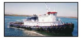
**File: TG39149 Tug - Twin Screw:** 100.0' loa x 30.1' beam x 12.4' depth. Built in 1977 by Chromalloy American Corp. U.S. flag. GRT: 182. ABS Loadline exp. Aug. 2021. FO: 40,000g. FW: 14,700g. Winch: None. Main Engines: 2 x EMD 16-645E2 total **3,900BHP**. 2 - 86" x 56" 4-blade FP props. Repowered 1982 / Orig. 567 blocks, bored out to 645s. **Bollard Pull: 32T**. Gensets: 2 - 60kW / GM6-71. AirCon. Galley. Harbor tug. Fitted with vertical capstan and H-bitt. **U.S. Gulf Coast.**
