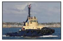
**File: TG47711 Tug - Azimuthing:** 111.3' loa x 35.5' beam x 17.7' depth. Built in 1986 by Australian Shipbuilding, Australia. Australia flag. GRT: 470. LR+100A1, +LMC, UMS SS due Nov 2021. Winch: Hagglund fwd. and aft. Main Engines: 2 x Daihatsu 8Z 280-ET total **4,747BHP**. 2 - Niigata Z-Peller props. **Bollard Pull: 43mt**. Gensets: Cummins. **Australia.**
