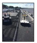
File: TB29755 / TB29754 Tank Barge – Inland (Two Available): 297.6' loa x 54.0' beam x 12.0' depth. Built in 1995 by Trinity Marine, Gulfport. U.S. flag. GRT/NRT: 1,619. USCG COI Lakes, Bays & Sounds & Limited Coastwise. Exp. Oct 2020. Capacity: 30,000bbl. U.S. Gulf Coast.
