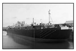
Stevenson hydraulic drive & pump system. **Vapor Recovery system**. Yokohama fender slides port fore & aft. Emergency tow wire. Panama chocks. Dry docked, painted & all certificates freshly renewed late 2018, including second five year Special Survey, etc. ITC Tonnage: 5,813G / 3,914N. Compatible tug side of JAK system from former tug may be made available for installation on new tug. **U.S. Gulf Coast.**
