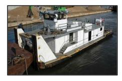
File: TP07065 Push Boat: 65.0' loa x 18.0' beam x 6.0' depth x 5.20' loaded draft. Built in 1971 by South Shore Marine Shipyard; Holland, MI. U.S. flag. GRT: 65. Main Engines: 2 x Cummins N14 total 700BHP. Inland river pushboat. Retractable wheelhouse. Highest fixed point 15.6'. U.S. Midwest.
