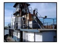
**File: TP14559 Push Boat:** 59.0' loa x 19.5' beam x 8.2' depth. Built in 1990 by Aiple Marine; Stillwater, MN. Rebuilt: 2002. U.S. flag. GRT: 77. Main Engines: 2 x CAT D348 **total 1,450BHP**. Last Overhauled: 2002. 2 - FP prop(s). Rebuilt 01/2002 by Alsem Industries. Genset(s): 2 - 40kW / GM3-71 (overhauled 2002). Quarters: 8. Galley. Totally rebuilt in 2002. Rewired. Upper Pilot house. Height of eye = 40'. **U.S. Gulf Coast. Prompt.**
