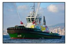
4.38m; Maximum draft: 5.40m. The CAT AVD TM system consists of a pair of dual input, continuously variable transmissions, located in the shaftlines between the main engines and the Z-drives. The AVDs can accept power from the CAT 3512 main engines, rated 1,765kW at 1,800RPM and/or from two 435kW hydraulic motors powered by a single CAT C32 auxiliary engine rated 1,081kW at 2,100RPM. The power is delivered to two CAT MTA 627 FP Z-drive units with 2.7 metre diameter fixed pitch propellers.
