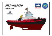
**Med Marine**, has signed a new deal with **Kenya Ports Authority** (KPA) for a brandnew RAstar 4200 (MEDA42120) tugboat. The new RAstar 4200 with a bollard pull of 120 tonnes, will be amongst the most powerful tugs Robert Allan Ltd. has ever designed. Technical details: Length o.a.: 42.0 m; Beam, moulded: 16.0 m; Depth, least moulded: 6.4 m; Draft, maximum: 7.2 m; Bollard pull 120 tonnes; Fuel oil: 500 m3; Fresh water: 60 m3; and Complement: 18 crew.
