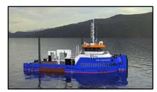
tug is equipped with a 4-point mooring system and spudleg system for maximum stability. Features on the 250m2 aft deck include a Heila 280 and a 120mt deck cranes, a moonpool and a 100mt AHT winch.
