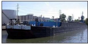
**Heated asphalt barge**. Raised trunk. 5 cylindrical cargo tanks. Double hull. Double chine bow, raked stern fitted with skegs & **notch for tug**. 8.0 million BTU/h vapor-liquid phase heater. Outlet temperature 385deg F. Barge has worked in fresh water since 1990. Unmanned barge. Approved for Grade E combustible materials in molten form. Contact Marcon for price ideas and further details. **U.S. Great Lakes.**
