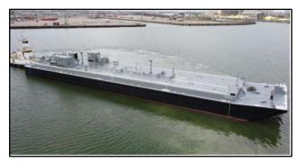
HPU house, hydraulic cargo hose handling cranes, and an air conditioned tankermans shed.
