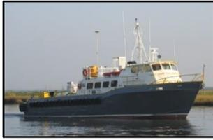
**File: CB09003 Crew Boat:** 90.0' loa x 21.0' beam x 7.0' depth x 5.50' light draft x 6.00' loaded draft. Built in 1972 by Breaux's Bay Craft. Foreign flag. GRT: 100. Deck Cargo: 25T on 36' x 17' clear deck. FO: 2,000g. FW: 300g. Main Engines: 3 x GM 12V71TI total 1,530BHP. **Speed about 20kn** on 75gph. Genset(s): 2 - 30kW / GM3-71. Firefighting: 1,000gpm fire monitor topside. 150g foam tank. Quarters: 10. AirCon. Galley. **Passengers: 65.** All aluminum. Vessel is working. **Caribbean.**
