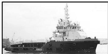
(E), +AMS, +DPS-1. Accommodations can provide 42 persons. The AHTS “*Errington Tide*” (pictured left) was sold to **Ships & Boats Oil Services** in Egypt. They renamed the vessel as the “*Sea Bird*”. The Conan Wu design AHTS vessel was built in 2009 and is classed ABS +A1, Towing, FiFi-1, OSV AH, (E), +AMS, +DPS-1, Unrestricted Service. It measures 197' x 52.5' x 19.7' x 16.4' loaded draft; is driven by two Niigata 6MG28HX main engines totaling 5,000BHP driving two Kamome
