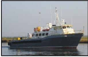
**File: CB09003 Crew Boat:** 90.0' loa x 21.0' beam x 7.0' depth x 5.50' light draft x 6.00' loaded draft. Built in 1972 by Breaux's Bay Craft. Foreign flag. GRT: 100. Deck Cargo: 25T on 36' x 17' clear deck. FO: 2,000g. FW: 300g. Main Engines: 3 x GM 12V71TI total 1,530BHP. **Speed about 20kn** on 75gph. Genset(s): 2 - 30kW / GM3-71. Firefighting: 1,000gpm fire monitor topside. 150g foam tank. Quarters: 10. AirCon. Galley. **Passengers: 65.** All aluminum. Vessel is working. **Caribbean.**
