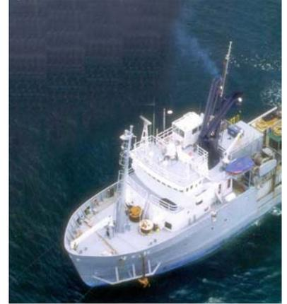
Marcon also arranged a 3 month charter (with options) for the 215' x 45' DP Class II Vessel 'Argo II' (ex-Augustea Otto, ex-Maersk Plotter) powered with twin MAK diesels providing 3,000BHP plus bow & stern thrusters. Vessel was built in 1978 BV Schp. Waterhuizen and converted to current configuration in 2000. The vessel is now engaged in underwater support in the Mediterranean region, and will become available again towards the end of 2002. Call Marcon for further details and charter inquiries.
