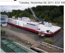
This unique hover or air cushion barge (ACB) was designed to hover about 5' above the surface while carrying about 450 tons of deck
