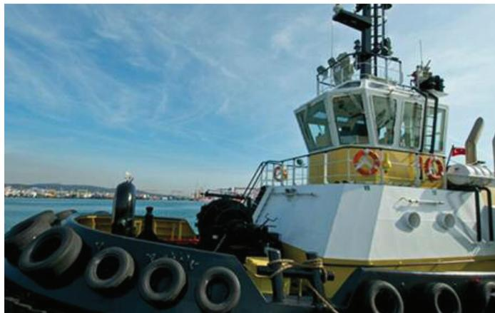
The RINA C+ Hull & Machinery classed tug is fitted with Rolls-Royce Rauma Brattvaag hydraulic towing winches fore and aft, Data hydraulic 8" towing pins and a Data hydraulic 45 tonne SWL quick-release tow hook. Two Volvo-Penta diesel generators provide electrical power.
