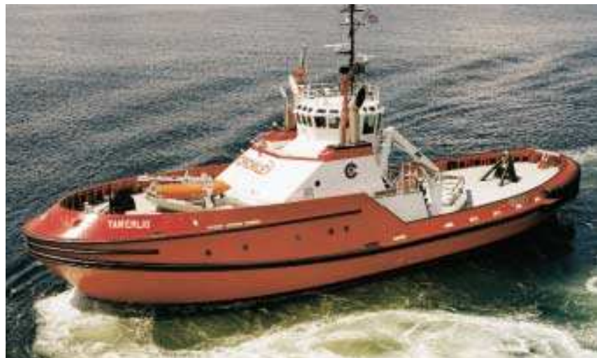
Figure 2: Voith Water Tractor Tan'erliq of 6,920 kW
