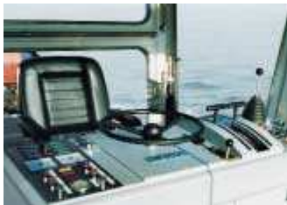
Figure 10: VSP control stand in the wheel house
